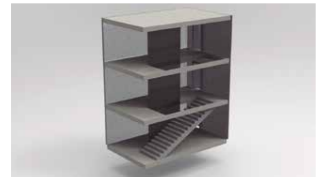
PHASE 2 Demolition of the first section of the stairs without the neighbours having to leave their homes. The neighbours will be informed of the length of time they are without stairs (4 hours).
